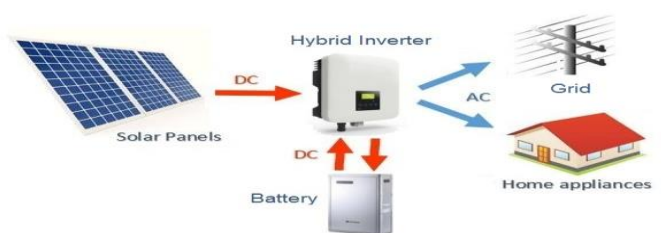
Figure 22 Illustration of the input & output currents to the Hybrid Inverter.
